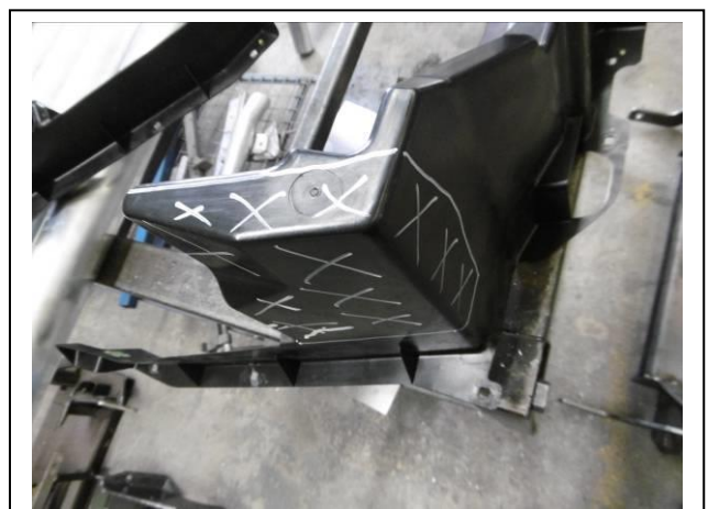
Figure 10: Trim line R/H air scoop
