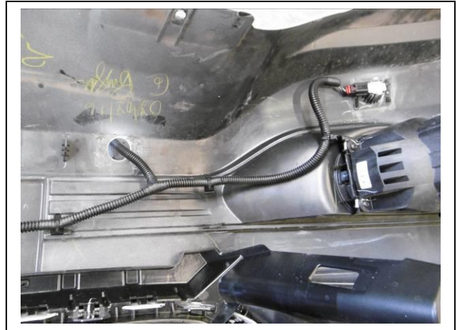
Figure 12: Relocate sensor and wiring into protection bar.
