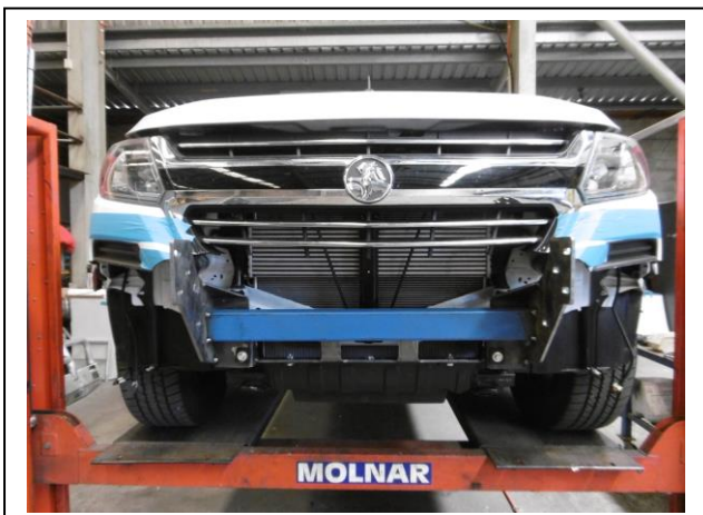
Figure 9: Steel mount installed
