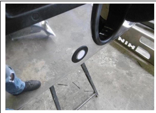
Figure 13: Sensor fitted into housing in protection bar.
