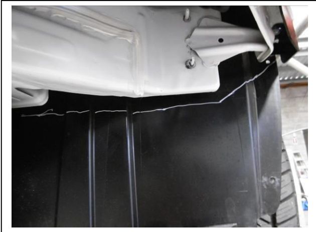
Figure 5: Trim line L/H liner
