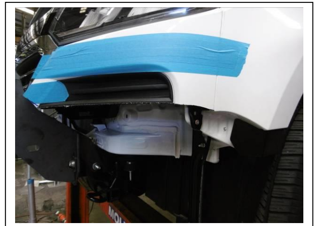
Figure 14: Cut bumper under headlight across to grille
