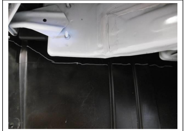
Figure 6: Trim line R/H liner
